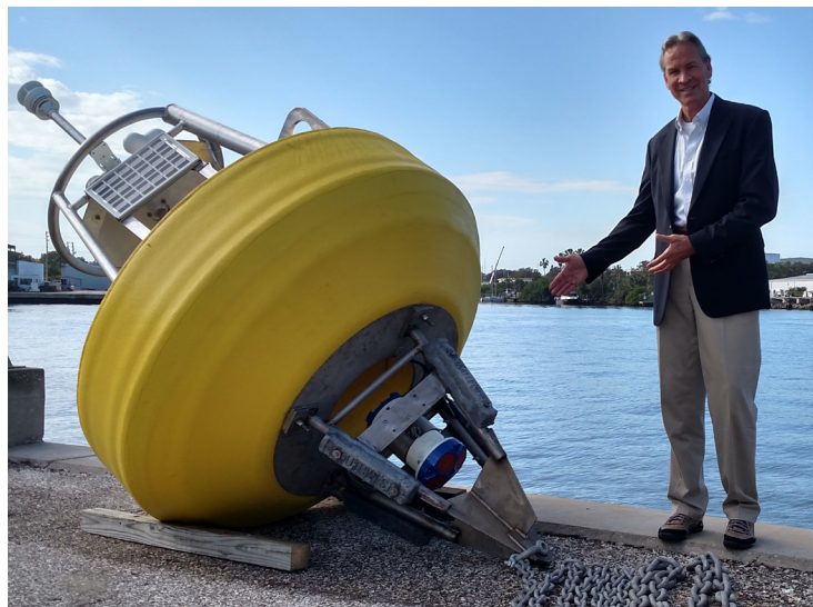
Underside of buoy, with OBS501 Smart Turbidity Meter mounted on left side
