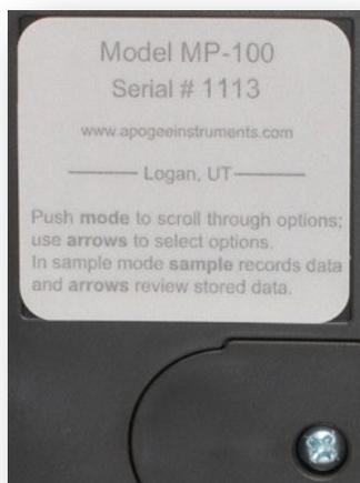
Sensor model number and serial number are located on a label on the backside of the handheld meter.
