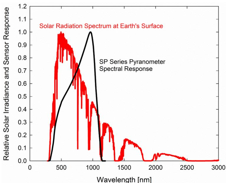
Spectral response of Apogee silicon-cell pyranometers compared to solar radiation spectrum at Earth's surface. Silicon-cell pyranometers, such as Apogee SP series, are only sensitive to the wavelength range of approximately 350-1100 nm, and are not equally sensitive to all wavelengths within this range. As a result, when the spectral content of solar radiation is significantly different than the spectrum that silicon-cell pyranometers were calibrated to, spectral errors result.
