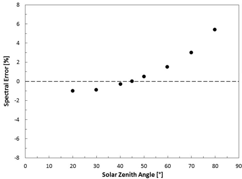
Spectral error for Apogee pyranometers as a function of solar zenith angle, assuming calibration at a zenith angle of 45°.
