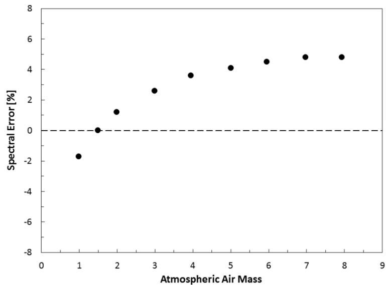
Spectral error for Apogee pyranometers as a function of atmospheric air mass, assuming calibration at an air mass of 1.5.
