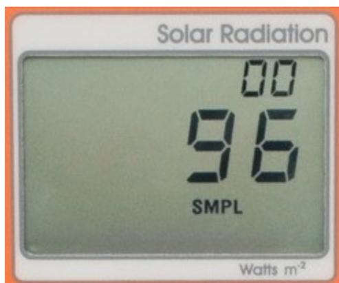
The LCD display consists of the total number of logged measurements in the upper right hand corner, the real-time irradiance value in the center, and the selected menu options along the bottom.
