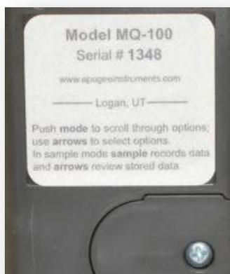
Sensor model number and serial number are located on a label on the backside of the handheld meter.
