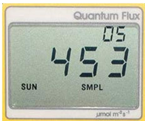
The LCD display consists of the total number of logged measurements in the upper right hand corner, the real-time PPF value in the center, and the selected menu options along the bottom.
