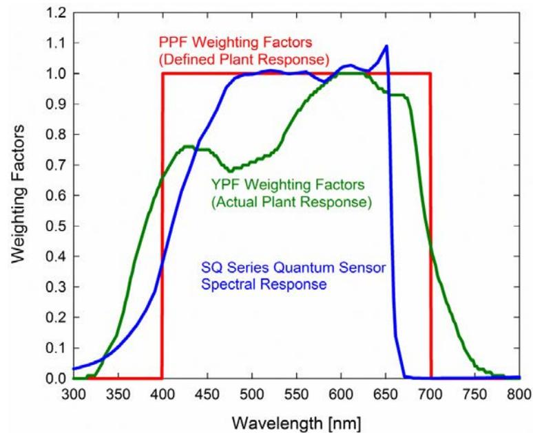
Radiation weighting factors for PPF (defined plant response to radiation), YPF (measured plant response to radiation), and Apogee quantum sensors (sensor sensitivity to different wavelengths of radiation).
