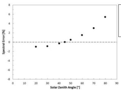
Spectral error for Apogee SP series pyranometers as a function of solar zenith angle, assuming calibration at a zenith angle of 45°.
