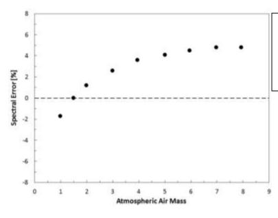
Spectral error for Apogee SP series pyranometers as a function of atmospheric air mass, assuming calibration at an air mass of 1.5.
