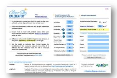
Clear Sky Calculator for pyranometers. Site data are input in blue cells in middle of page and an estimate of total shortwave radiation is returned on right-hand side of page.
