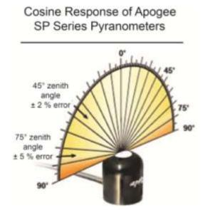
Directional, or cosine, response is defined as the measurement error at a specific angle of radiation incidence. Error for Apogee silicon-cell pyranometers is approximately  $\pm$  2 % and  $\pm$  5 % at solar zenith angles of 45° and 75°, respectively.
