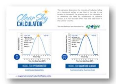
Homepage of the Clear Sky Calculator. Two calculators are available: One for pyranometers (total shortwave radiation) and one for quantum sensors (photosynthetic photon flux).
