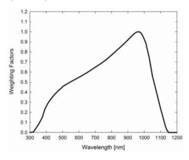
Spectral response estimate of Apogee silicon-cell pyranometers. Spectral response was estimated by multiplying the spectral response of the photodiode, diffuser, and adhesive. Spectral response measurements of diffuser and adhesive were made with a spectrometer, and spectral response data for the photodiode were obtained from the manufacturer.
