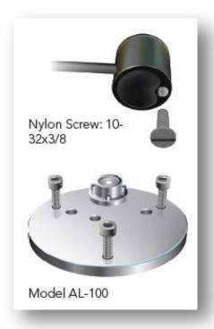
To minimize azimuth error, the sensor should be mounted with the cable pointing toward true north in the northern hemisphere or true south in the southern hemisphere. Azimuth error is typically less than 1 %, but it is easy to minimize by proper cable orientation.
