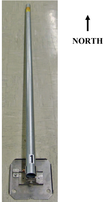
FIGURE 3-4. Mast Section 1 oriented on base
