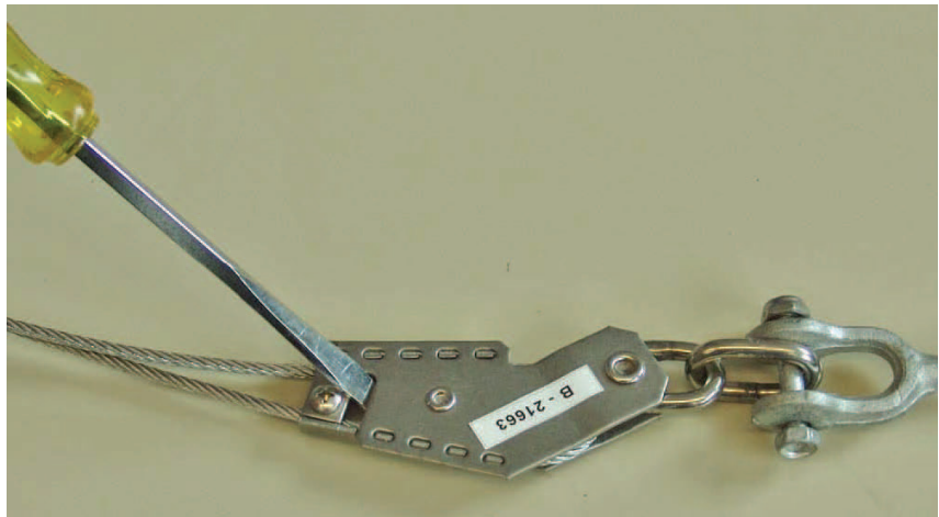
FIGURE 3-28. Adjusting cable through wedge clamp
