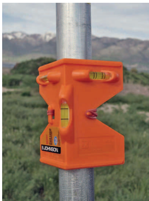
FIGURE 3-30. Post level ensures vertical mast
