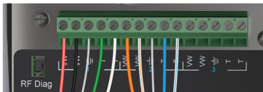
Figure 7-2. Typical vibrating-wire sensor wire colors and connections
