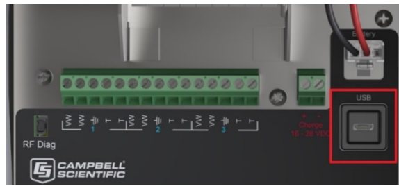
Figure 7-4. CRVW3 USB connection location
