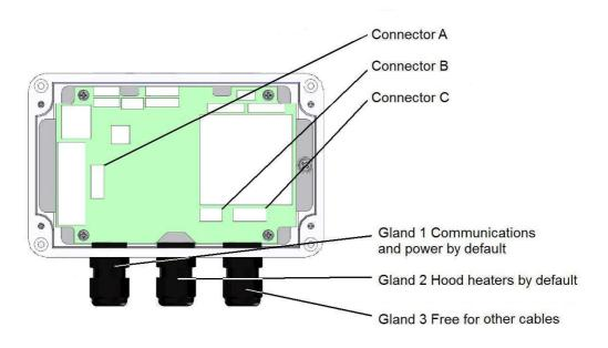
A configuration cable, part number 010817, is available from Campbell Scientific that plugs directly into connector B, in place of the normal connector and cable. The configuration cable is fitted with a 9-way D connector for use with a PC serial port or USB to serial adaptor.
