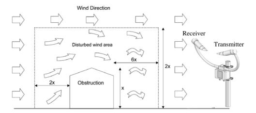
In order to reduce the service frequency with the unit, the CS120A should be placed away from sources of contamination, in the case of roadside monitoring; larger mounting poles can be used. More regular maintenance will be required when the instrument is placed in areas where contamination is unavoidable or where measurements may be safety critical.
