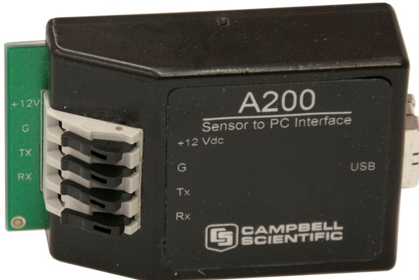
FIGURE 3-1. A200 Sensor-to-PC Interface
