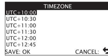
Time zones from UTC-12 to UTC+14 are available. Use to select a time zone and press . To exit without making changes, press .
