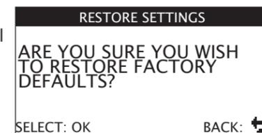
This step cannot be undone. If the unit is inadvertently set to factory defaults, all settings will need to be restored manually through the previous menus.
