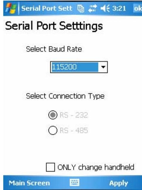
FIGURE 1-6. Dialog Box for Changing Baud Rate
