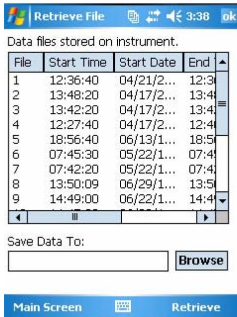
7. Wait for the progress bar to disappear and examine data as a plot or test file (Section 1.16—Graphing).
