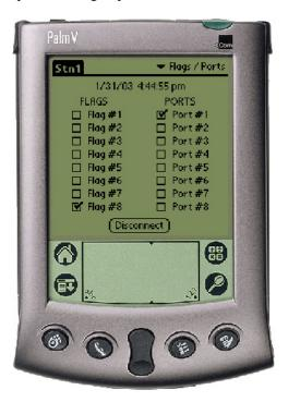
To change the state of a flag or port, touch the box for that flag or port. There may be a short delay between when the box is touched and when the state of the flag or port appears to change.
