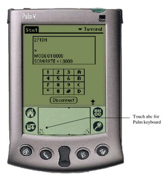
For all dataloggers except the CR1000, CR200, CR800/850, and CR3000, the datalogger's keyboard/display keypad is depicted on the *Terminal* window. The Palm device's grafitti pad or keyboard can also be used to enter characters. For CR1000, CR800/850, CR200, and CR3000 dataloggers, there is no keyboard/display depicted, so the graffiti pad or keyboard must be used.
