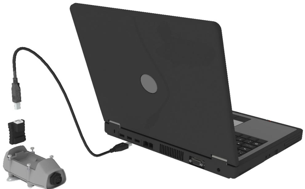
FIGURE 6-2. Connecting a computer to a sensor
