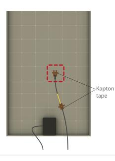
Kapton tape is used to fasten the sensor to the back of a solar panel and for cable strain relief when the temperature may exceed 70°C.
