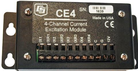
The number of 229 sensors measured by one datalogger can be increased by connecting a CE4 or CE8 to one or more AM16/32-series multiplexers<sup>2</sup>. Up to four multiplexers can be connected to the CE4, and up to eight multiplexers can be connected to the CE8.
