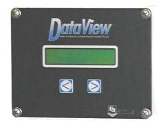
The CD294 supports mixed-array dataloggers—specifically the CR510, CR10X, CR23X and CR7. PC294 software is provided with the CD294. This software allows the customer to specify up to 18 input locations to display along with their descriptions and units. To conserve power, the CD294 automatically goes into a quiescent state when the customer hasn't pressed a button within two minutes.
