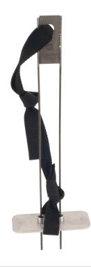
The CS650G makes inserting CS625 easier in dense or rocky soils. This tool can be hammered into the soil with force that might damage the sensor if the CS650G were not used. It makes pilot holes into which the rods of the sensors can then be inserted.
