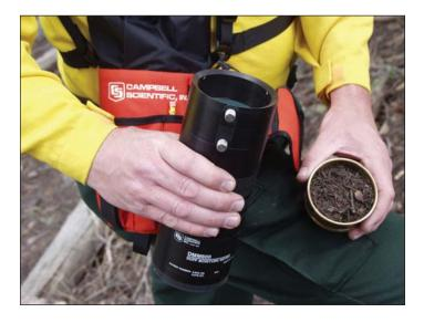
To measure duff water content, the sample is placed in the sample chamber and the compression knob is turned until an audible indicator signals the sample is properly compressed and the measurement is complete.
