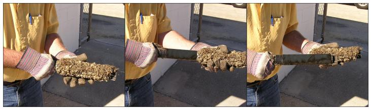
Two sleeve options are offered by Campbell Scientific. The three above photographs show the plastic sleeve being removed.
