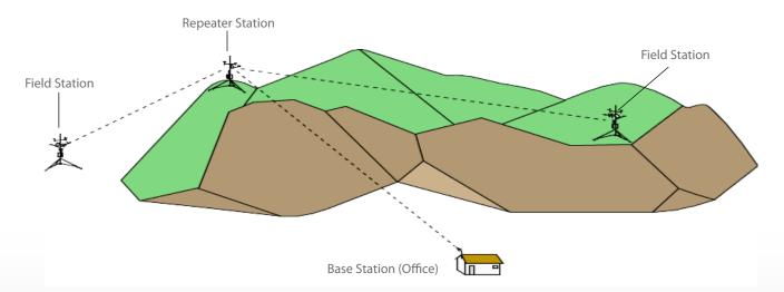
Our RF networks require line-of-sight transmission. The mountain in this drawing obstructs line-of-sight with the base station. Use of the repeater station allows the base station to receive data from the field stations.
