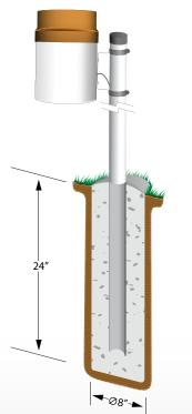
At left is a TE525 mounted onto a CM310 pole that is embedded directly in a concrete pad (-NP no pedestal base option).
