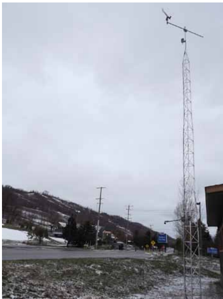
Campbell Scientific weather station installed immediately adjacent to Group Services building.
