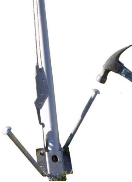
FIGURE 6-10. Staking the tripod feet
