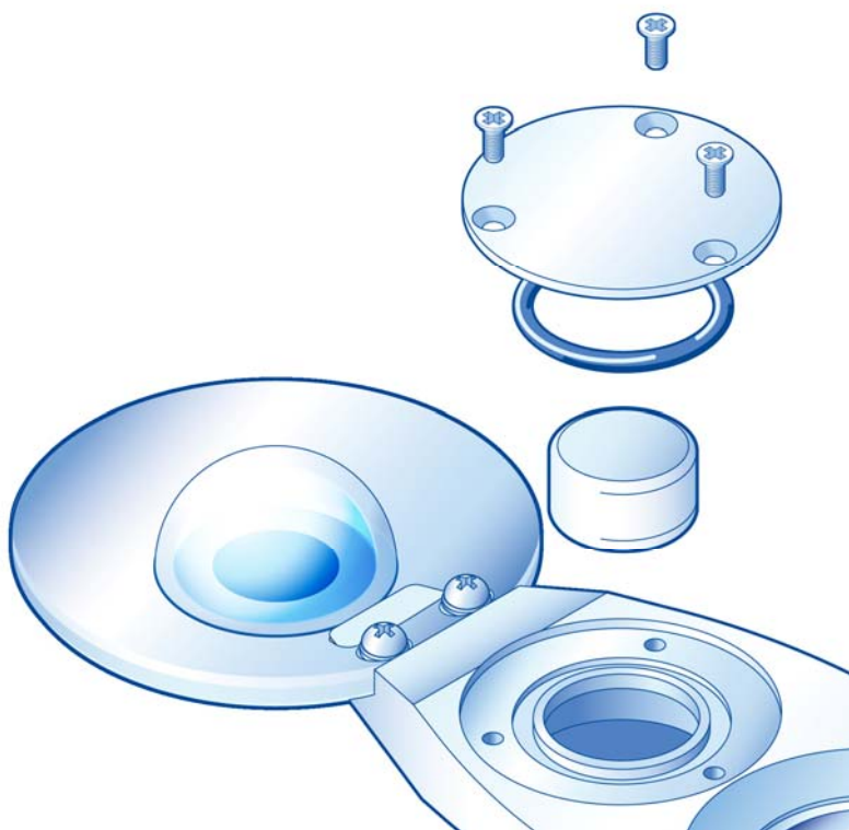
FIGURE 8-3. Replace Drying Cartridge Every Six Months (first replacement comes with CNR2)
