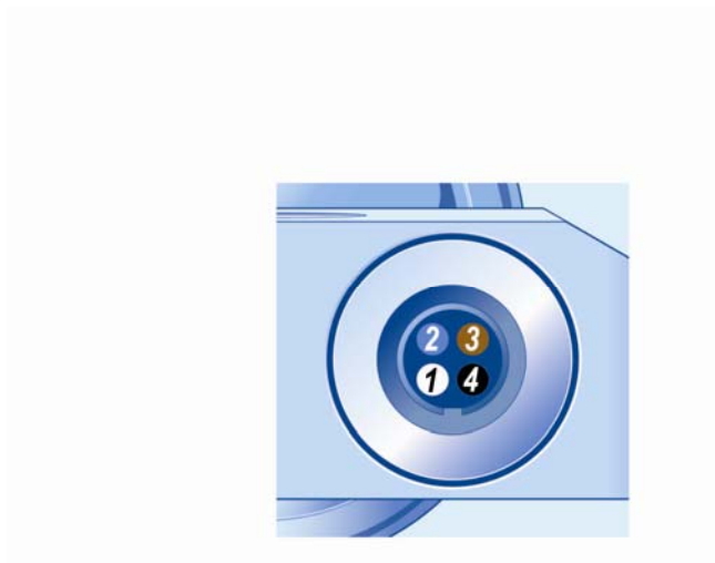
FIGURE 5-1. Pin Layout on Campbell Scientific Black Cable
