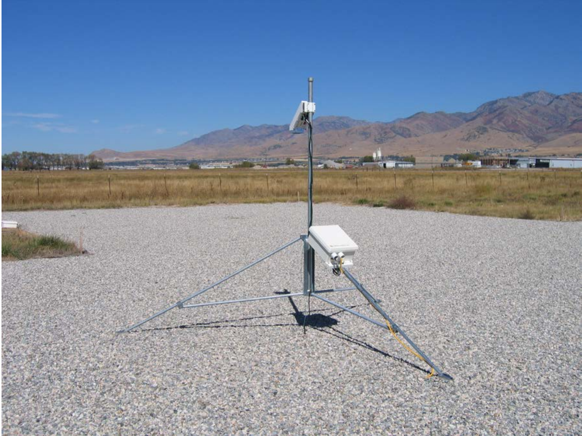
FIGURE G-1. CS110 2 Meter CM10 Tripod site
