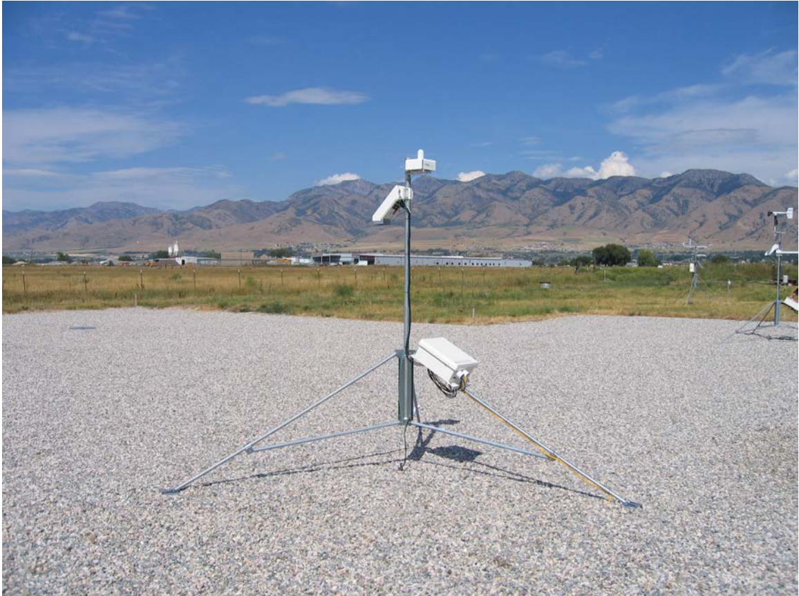
FIGURE H-1. Tripod CS110 and StrikeGuard
