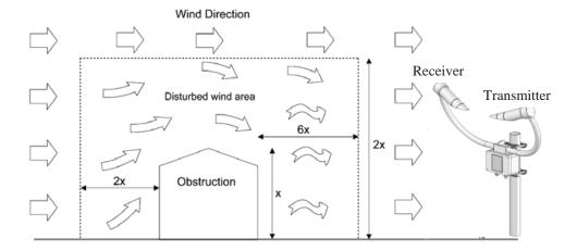
In order to reduce the service frequency with the unit, the CS125 should be placed away from sources of contamination, in the case of roadside monitoring; larger mounting poles can be used. More regular maintenance will be required when the instrument is placed in areas where contamination is unavoidable or where measurements may be safety critical.
