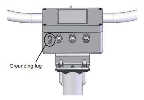
The CS125 must be properly grounded by taking a ground wire with a minimum cross sectional area of 6 mm<sup>2</sup> and maximum length of 5 m from the brass grounding lug in the lower face of the electronics enclosure to an adequate grounding point. The pole and foundations of a pole mounted installation will provide some basic lightning protection and protection against radio frequency interference and should also be correctly grounded.
