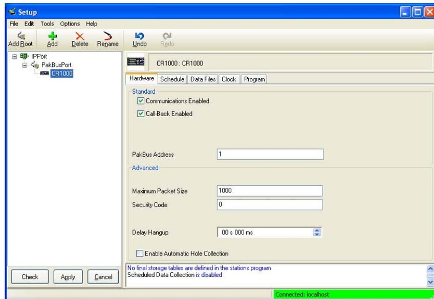
In some cases where signal strength is low, you may have to decrease the packet size of the CR1000. A recommended value of 400 bytes should be sufficient.
