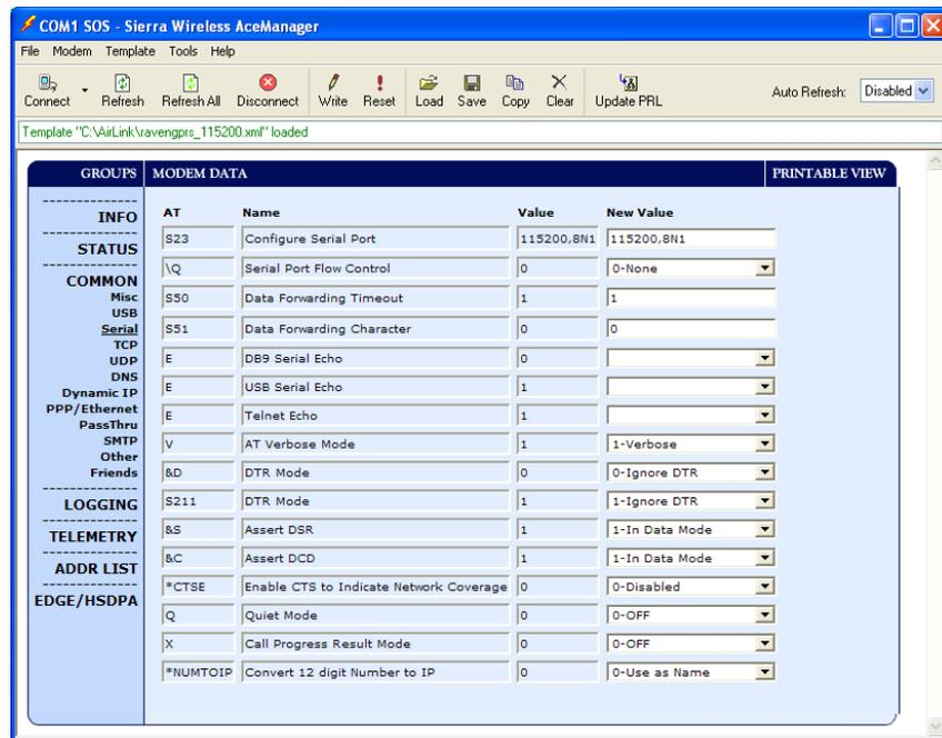
Connect to the modem with AceManager (Section 5.3). Select the “Serial” Group, and make sure the “AT Verbose Mode” is set to “Numeric” for use with the CR10(X), CR510, and CR23X dataloggers, or “Verbose” for other dataloggers (e.g. CR1000).
