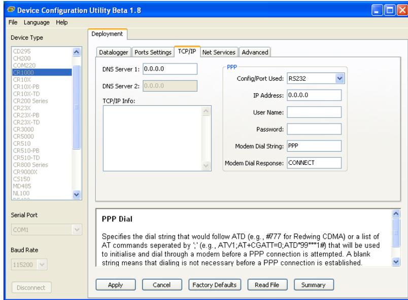
Using the Device Configuration Utility, select the “Net Services” tab. The “PakBus/TCP Service Port” default is 6785. This is the “Port” number that will follow the “IP address” for LoggerNet to communicate with the datalogger.
