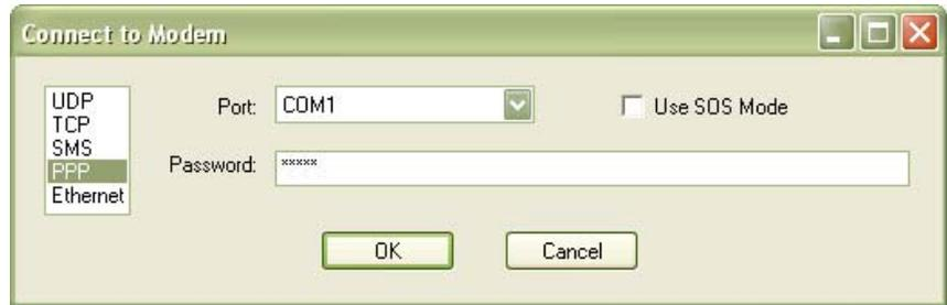
Make a note of the Device port (\*DPORT). The default is 12345 and we use 6785 in our template. Any valid port can be used. This is the port number used in LoggerNet to get to the datalogger.
