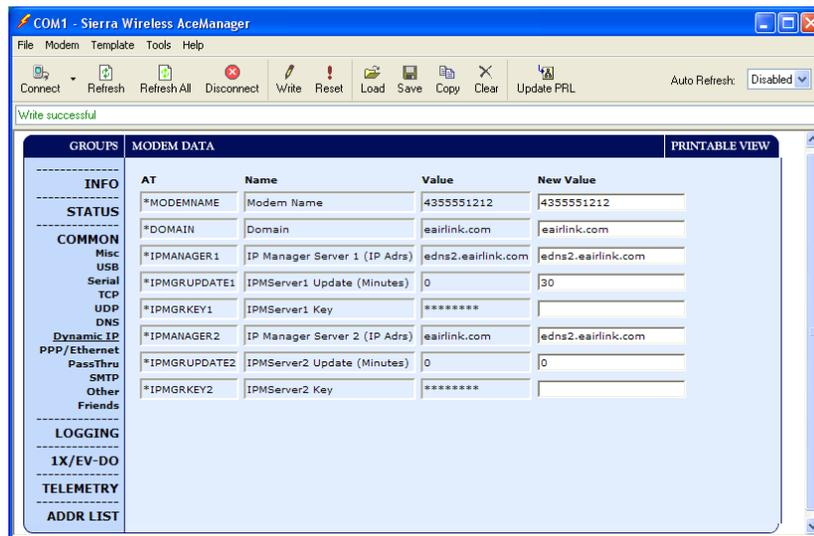
1. Modem name: A unique name for the modem (the 10-digit MSISDN number is recommended).
