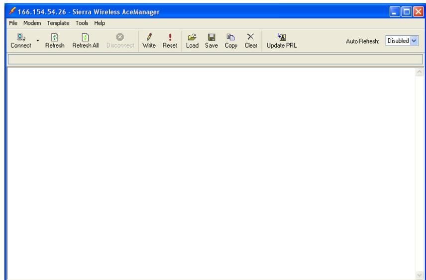
Click the **Connect** icon in the Configuration Panel to open the connection options dialogue box. Select PPP, and the COM port the modem is connected to. Do not change the Password (the default password is 12345). Click OK to continue.
