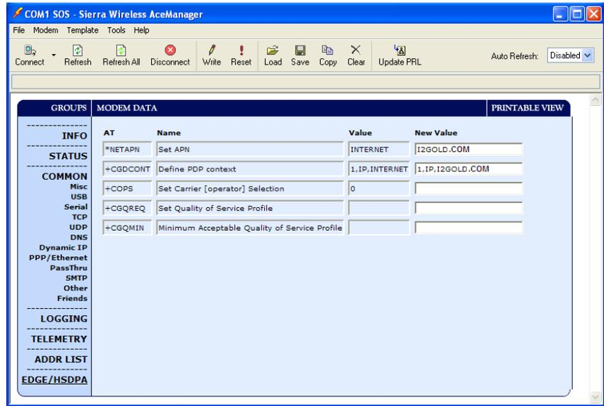
For a data account with the VPN.COM APN, enter the APN as shown in the following screen. The example is for an APN = "I2GOLD.COM".
