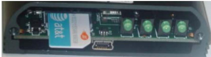
4. Replace the faceplate; the installation of the SIM is complete.
