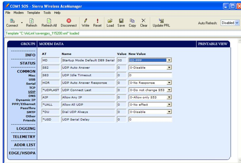
After the changes have been made, click the **Write** icon to save the changes in the modem.
