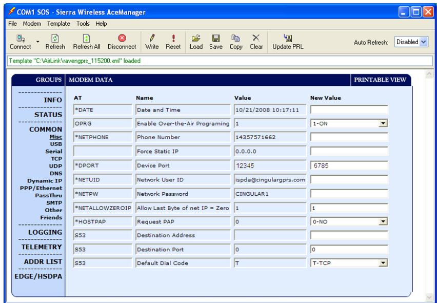
The Device Port gets changed from the default 12345 to 6785 when the template file is loaded into the modem (Section 5). The Device Port number gets entered with the IP address in LoggerNet (Section 6).
