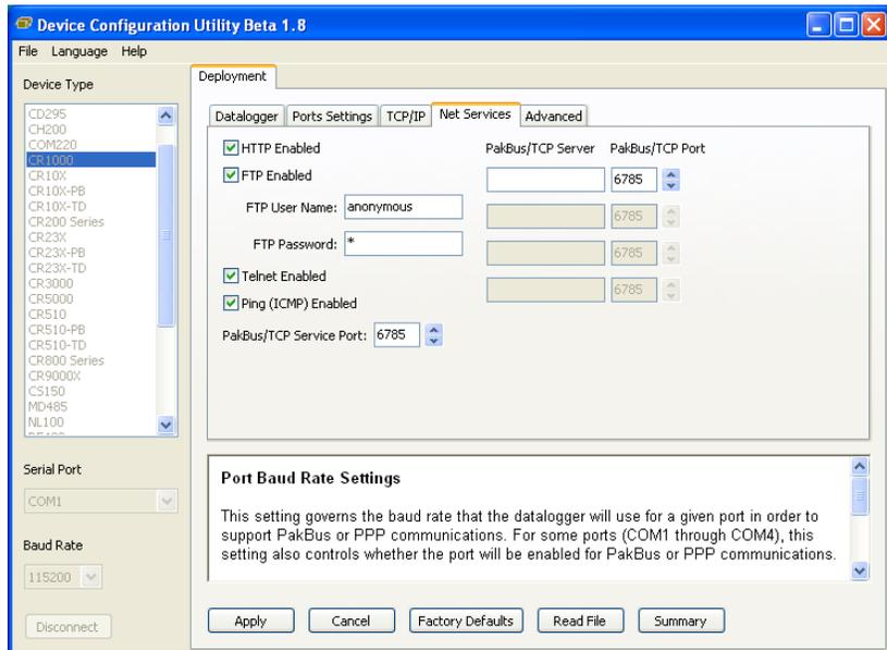
Using the Device Configuration Utility, fix the RS232 Baud Rate to “115200 Fixed” from the “Port Settings” tab.
