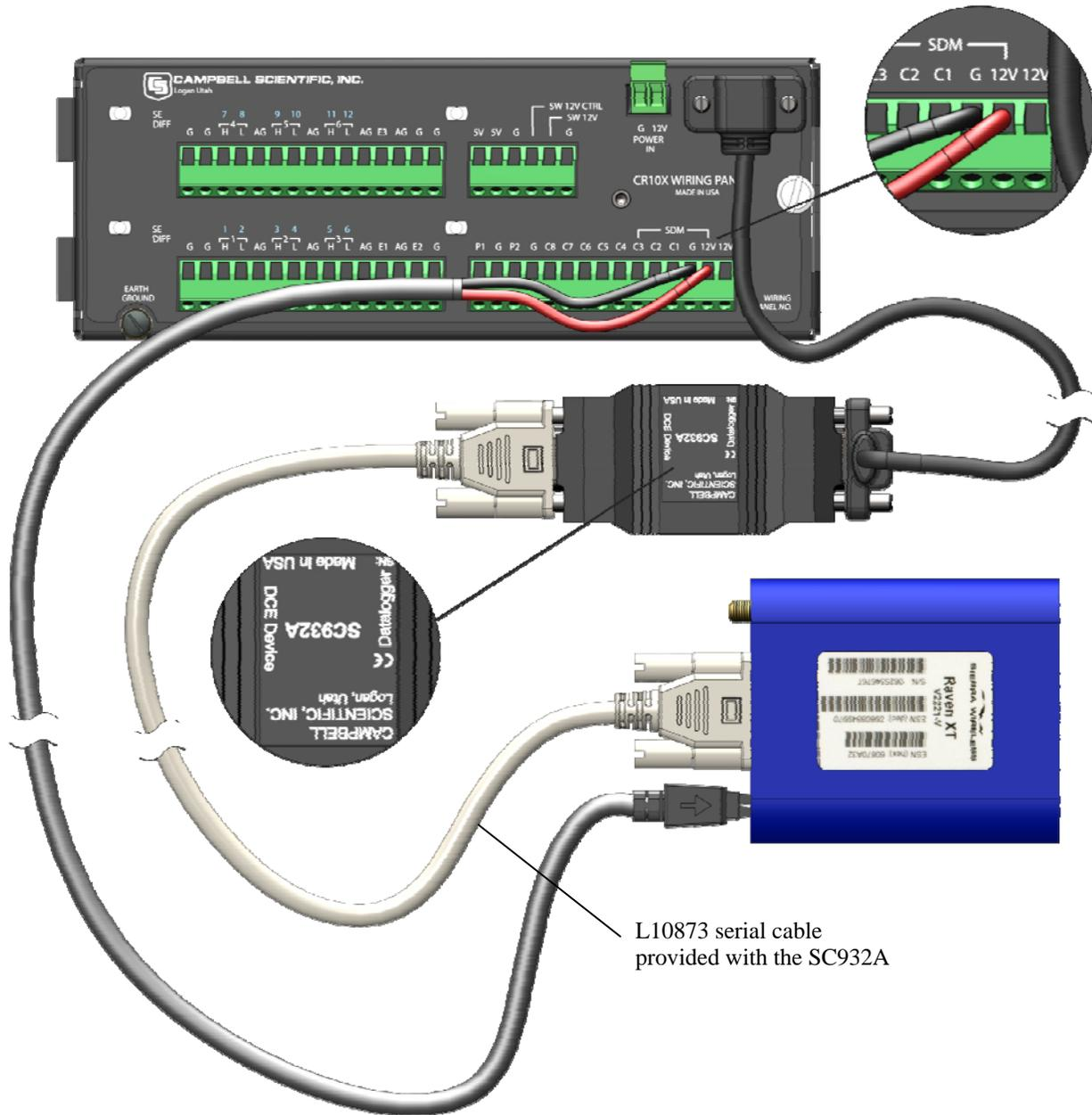
SC932A interface connects the modem to the CS I/O port; recommended for dataloggers with the Mixed-Array Operating System.
