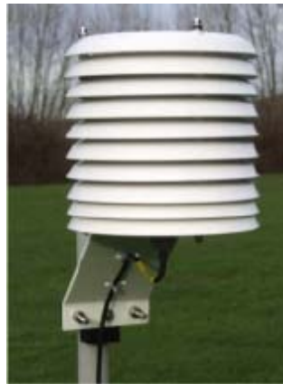
Figure 4. Met 20 Radiation Shield
