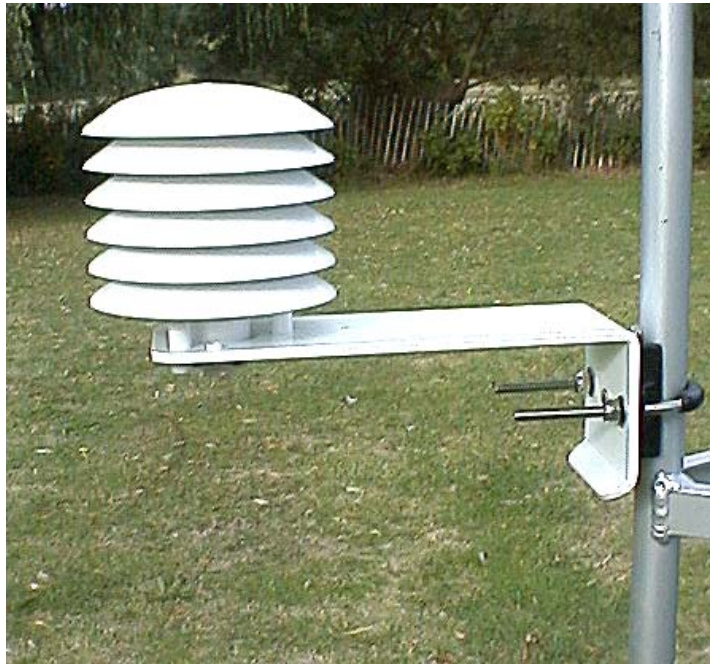
Figure 3. 41303-5 Radiation Shield and Mounting Arm
