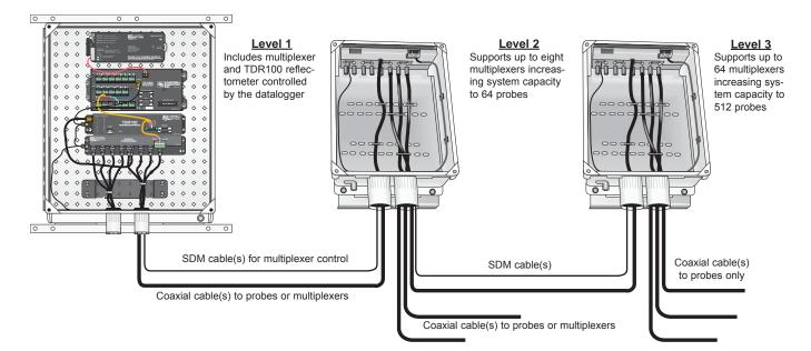
The system can use three multiplexer levels allowing up to 512 probes to be measured. The first level includes the TDR100 and one multiplexer. Up to eight coaxial cables connect to each multiplexer. The coaxial cables can be connected to TDR probes or the next level's multiplexers.
