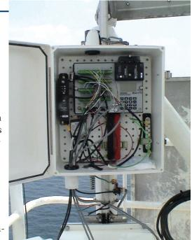
ments with the telemetry system on the tower results in a reliable, low-power solution. This solution enables consistent flow of data from the underwater sensors, and remote control of measurement frequency and power supply.
