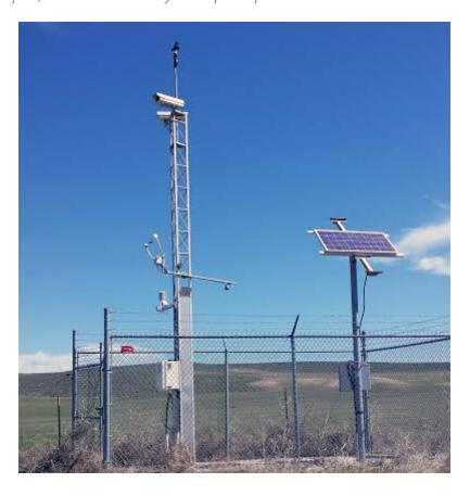
The Utah Department of Transportation (UDOT) operates a network of roadside weather stations across the state. A number of these were equipped with Campbell Scientific CS120 visibility sensors.
