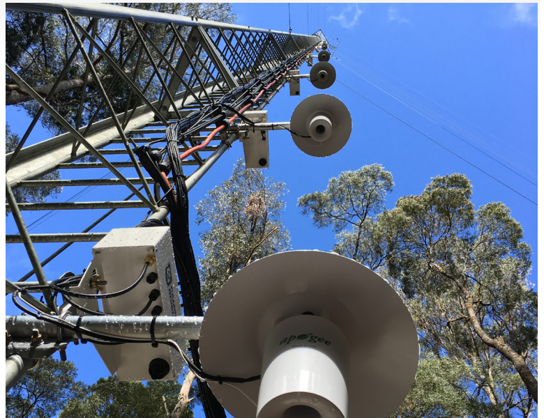
AP200 intakes and temperature probes on the Warra flux tower
