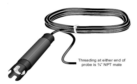
The CSIM11 and CSIM11-ORP are versatile sensors. manufactured by Wedgewood Analytical. The CSIM11 measures the full pH range and the CSIM11-ORP measures oxidation reduction potential (ORP). They are designed for submersion or insertion into tanks, pipelines, and open channels. Compatible dataloggers include our CR800-series, CR1000, and CR3000; one differential analogue input channel is required.
