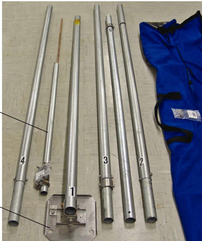
FIGURE 2.2-2. Mast Sections and Base
