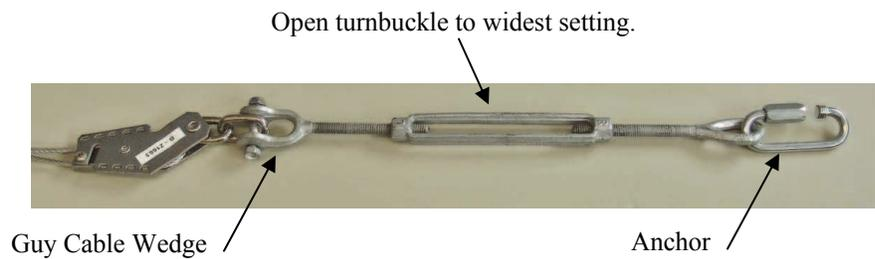
*FIGURE 2.4-6. Turnbuckle Fastened to Guy Cable and Anchor*
