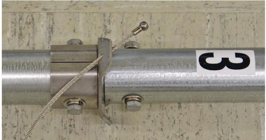
*FIGURE 2.2-11. Mast Section 3 and Guy Ring/Collar Assembly*
