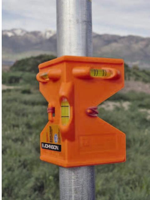
*FIGURE 2.5-2. Pole Level Ensures Vertical Mast*
