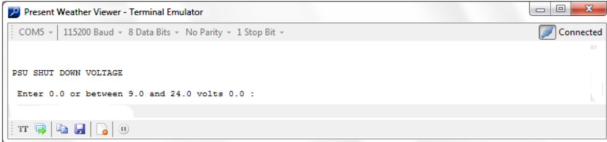
FIGURE 7-22. PSU shut down voltage menu
