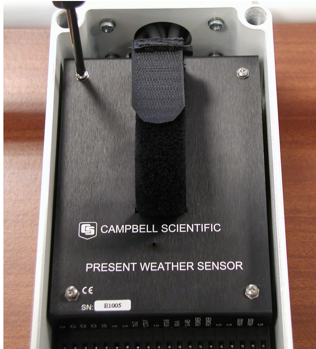
FIGURE 6-7. Removal of DSP cover.
