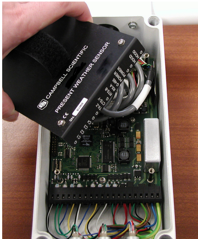
FIGURE 6-8. Exposing the DSP board.
