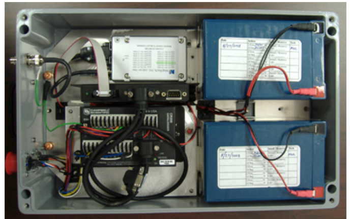
Datalogger, communication gear, and batteries in enclosure
