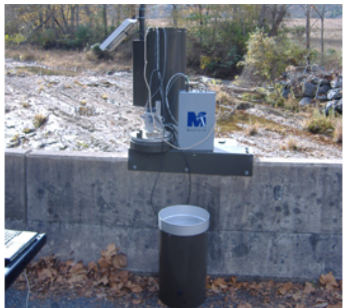
Datalogger, communication gear, and batteries in enclosure
