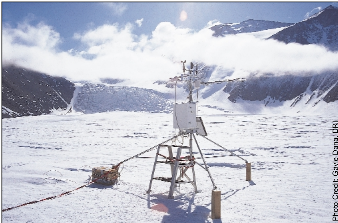
Eddy correlation station provides data for energy balance studies. (Canada Glacier, Taylor Valley, Antarctica).
