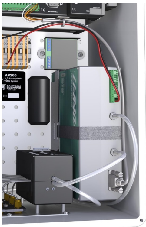
FIGURE 7-4. Installed IRGA in system enclosure
