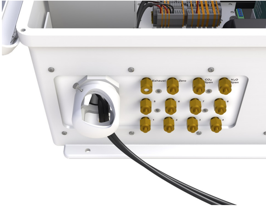
FIGURE 5-19. Cut-away view showing proper replacement of feedthrough cap
