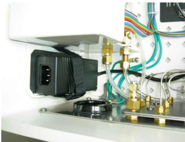
FIGURE 4-8. AC/DC power adapter kit installed in AP200
