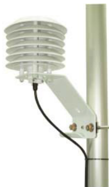
FIGURE 4-10. 107-L temperature probe mounted with radiation shield
