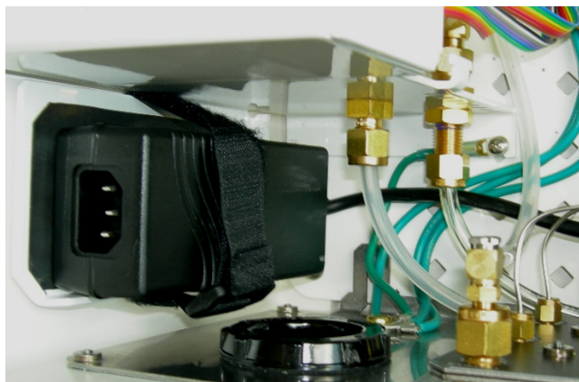
FIGURE G-1. Installation location of power adapter
