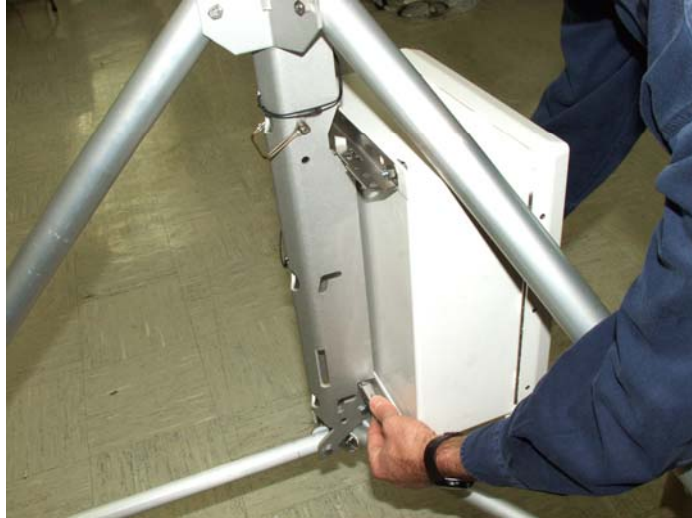
FIGURE 5-12. ENC 12/14 Enclosure Attached to the Tripod Base
