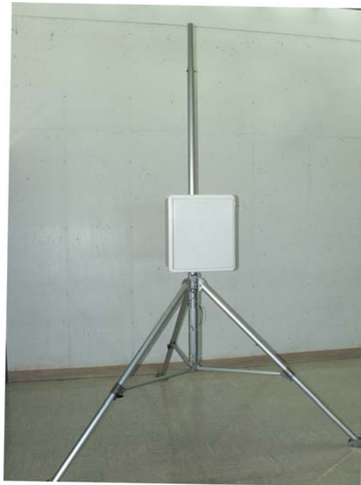
FIGURE 5-13. ENC 12/14 Enclosure Attached to the Mast
