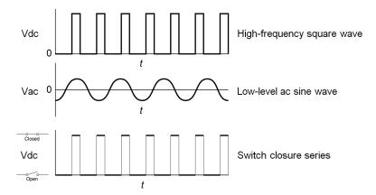
FIGURE 90: Switch Closure Pulse Sensor
