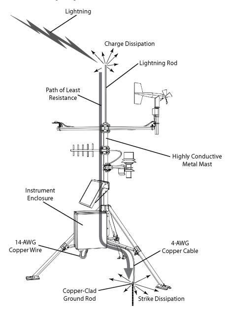
FIGURE 31: Lightning Protection Scheme
