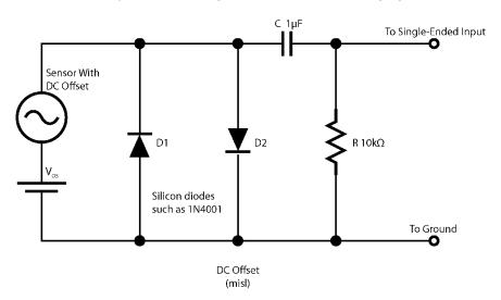
FIGURE 94: Input Conditioning Circuit for Period Averaging
