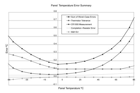
FIGURE 78: Panel Temperature Gradients (low temperature to high)
