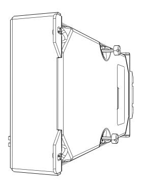
FIGURE 115: Loosen Retention Screws
