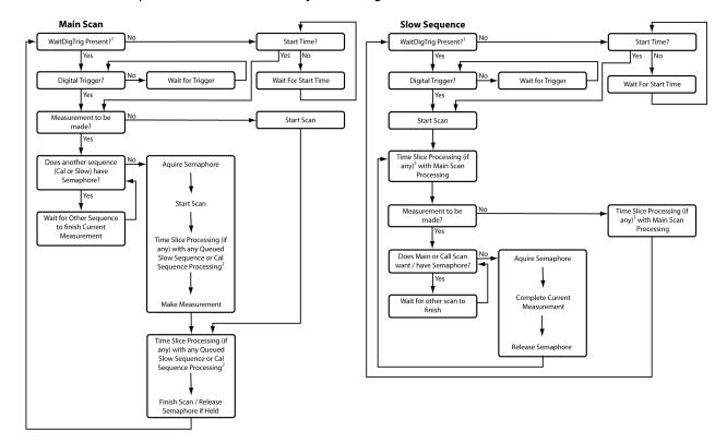
FIGURE 38: Sequential-Mode Scan Priority Flow Diagrams
