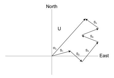
In figure Input Sample Vectors (p. 208), the short, head-to-tail vectors are the input sample vectors described by  $s_i$  and  $\Theta_i$ , the sample speed and direction, or by  $Ue_i$  and  $Un_i$ , the east and north components of the sample vector. At the end of data storage interval T, the sum of the sample vectors is described by a vector of magnitude U and direction  $\Theta_U$ . If the input sample interval is t, the number of samples in data storage interval t is t in t
