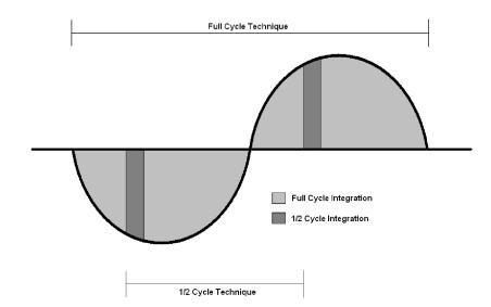
FIGURE 85: Ac Power Noise Rejection Techniques
