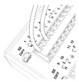
FIGURE 19: Analog Sensor Wired to Differential Channel #1
