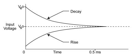
FIGURE 86: Input voltage rise and transient decay
