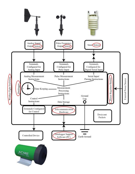
FIGURE 15: Data Acquisition System — Overview
