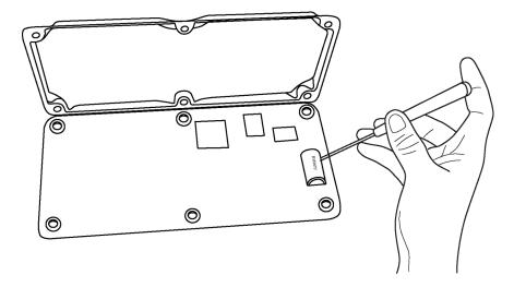
Remove the lithium battery by gently prying it out with a small flat point screwdriver. Reverse the disassembly procedure to reassemble the CR1000. Take particular care to ensure the canister is reseated tightly into the three connectors.
