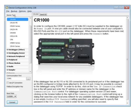
FIGURE 33: Device Configuration Utility (DevConfig)
