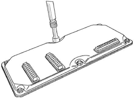
Remove six nuts, then open the clam shell.
