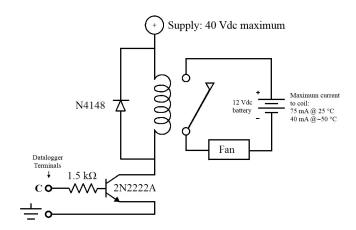
FIGURE 99: Power Switching without Relay
