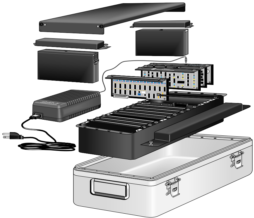
FIGURE OV1-1. CR9000 Measurement and Control System
