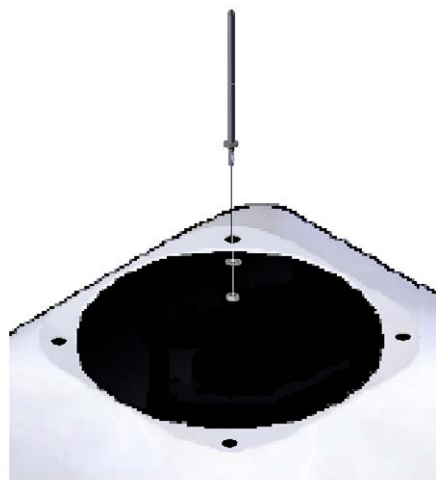
Fig 4.11 Attaching Bird Spikes to the CS135 cowl
