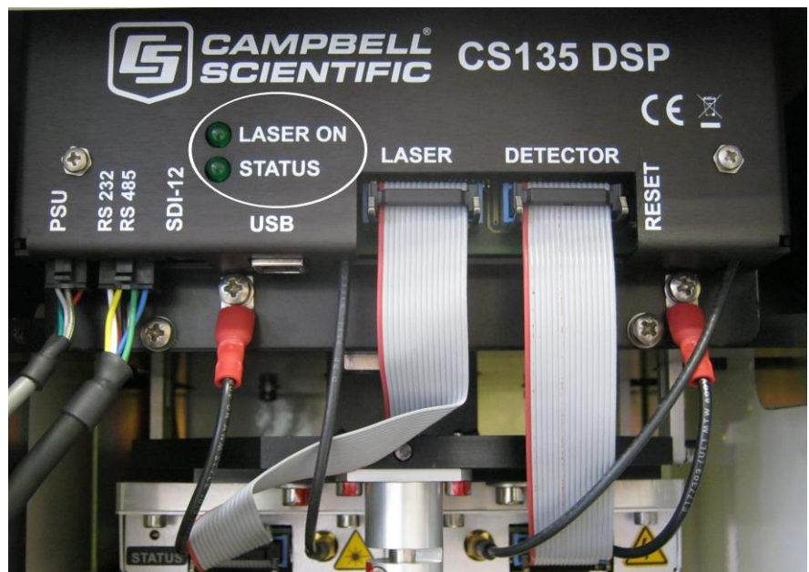
Fig 7.3 Diagnostic LED indicators
