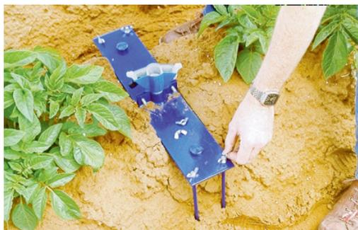
Lift both sections of the stabilization brace to clear the threads of the stabilization brace pins.
