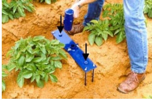
The stabilization brace should be firm to the ground without causing significant soil compression.
