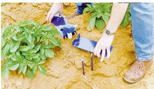
Continue inserting the probe into the ground with gentle blows of the sledgehammer using the EasyAG™ dolly until the base of the top cap is level with the ground. This will place the top sensor at 10 cm (3.9 inches) below the ground surface.
