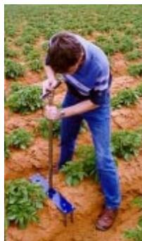
Using a sledgehammer beat the auger into the ground all the way. Ensure accurate blows are made such that lateral deflection of the soil sampler is minimized. Do not compress the soil with the final blow.
