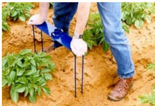
Using a sledgehammer alternately beat the stabilization brace at the points provided to force it closer to the ground. Do not beat continuously on any one side in advance of the other. The aim is to achieve a situation where the pins are near parallel in the ground.
