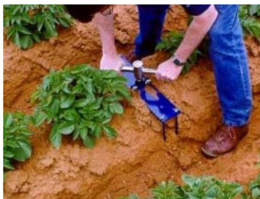
Carefully lift the AMS soil sampler directly out of the ground. If you experience difficulties at this point, remove the soil sampler in stages, or obtain extra assistance to avoid back injury. To remove the soil collected in the soil sampler, simply beat on its side with the hand or foot. The design is such that the soil core taken is slightly compressed, and of a lesser internal diameter than the soil sampler itself. Deposit this soil away from the probe site.
