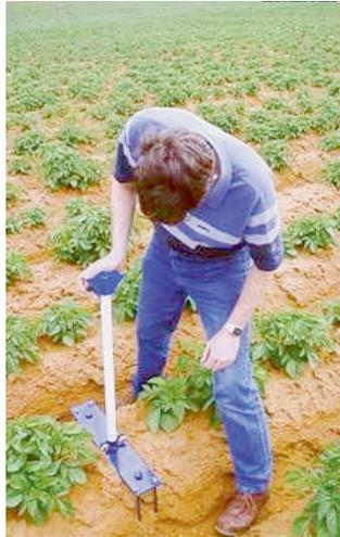
As the probe enters the prepared hole in the soil, it shaves off a residue that is eventually stored in the cutting tip at the base of the hole.
