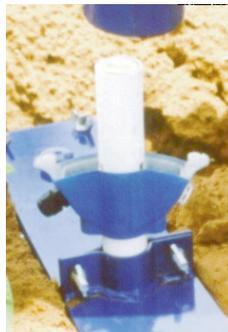
Remove all of the stabilization brace wing nuts.
