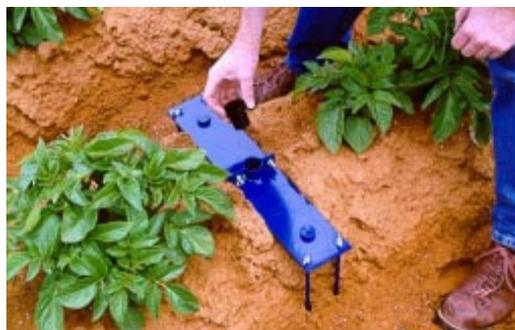
Put the soil sampler polyguide in place. The stabilization brace is now ready for insertion of the AMS soil sampler. Refer below from Step 5: Preparing the hole as for raised soil bed installation.
