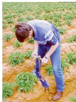
Remove the auger polyguide.
