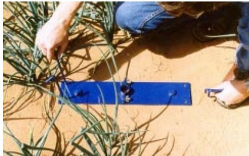
Drive the stabilization brace pins all the way into the ground using a sledgehammer. The stabilization brace should be in firm contact with the soil without compressing it significantly.
