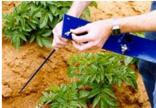
Place the assembled stabilization brace on the ground directly above the required position of the probe. Apply gentle pressure directly down onto the stabilization brace to force the pins into the ground.
