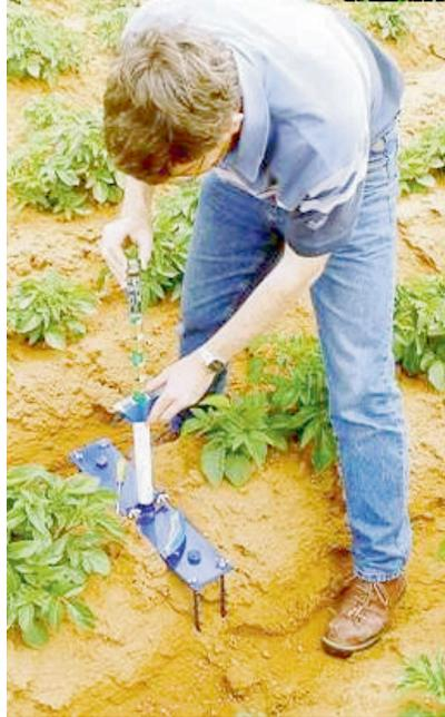
Insert the EasyAG™ dolly into the top cap and position it on top of the internal access tube.
