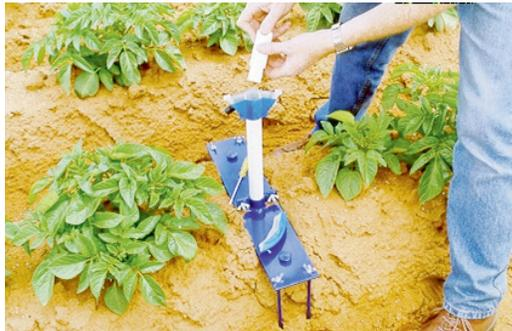
Continue inserting the probe using a sledgehammer until there is a 2.5 cm (1 inch) gap between the base of the top cap and the edge of the stabilization brace tube guide.
