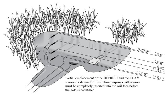
FIGURE 6-1. Placement of sensors
