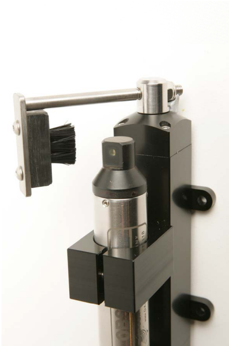
Photo 1. Mounting the OBS3+ in the Hydro-Wiper clamp
