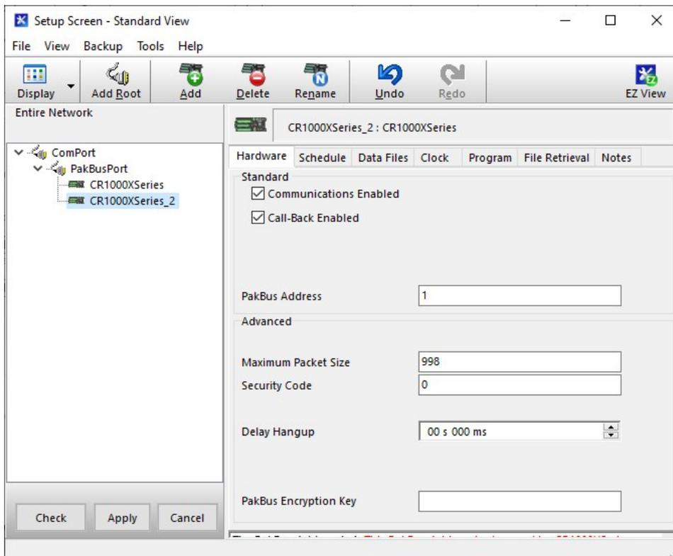
Figure B-2. *LoggerNet PakBus networking setup*
