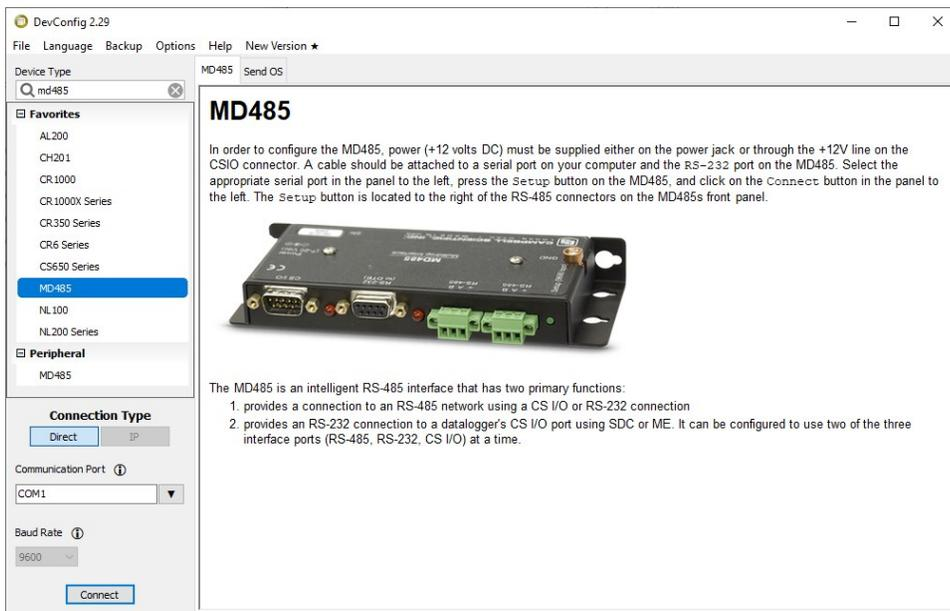
Figure 5-2. MD485 setup using *Device Configuration Utility*
