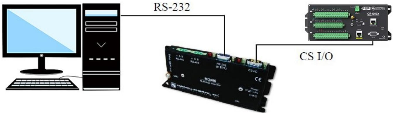
Figure 5-3. RS-232 to CS I/O conversion
