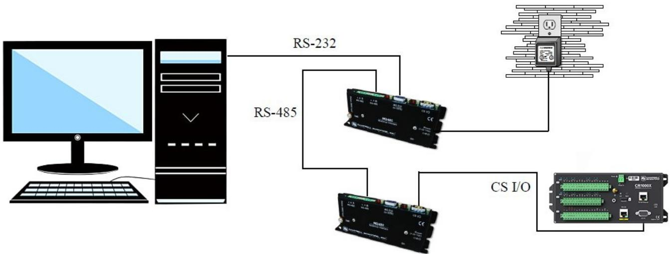
Figure 5-4. Long distance RS-232 to CS I/O conversion
