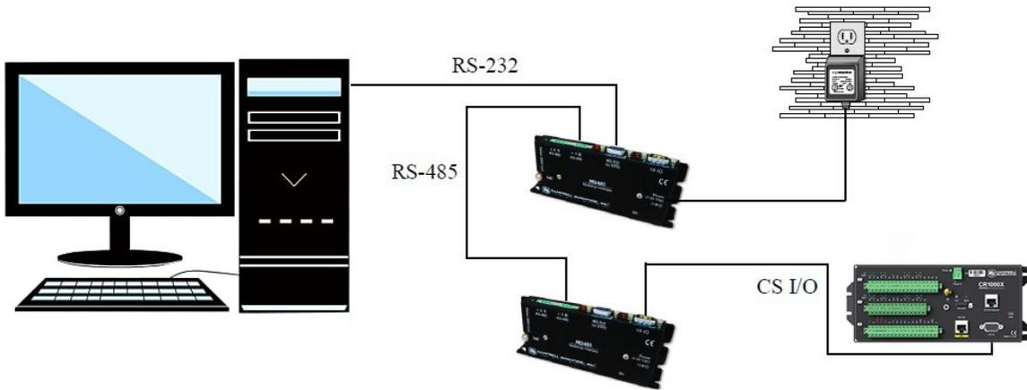
Figure 4-1. MD485 basic point-to-point network
