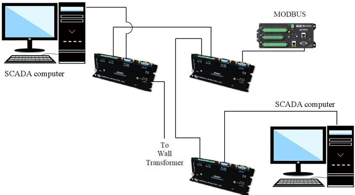
Figure 5-5. Transparent point-to-multipoint network
