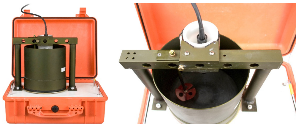
FIGURE 8-4. Portable sediment suspender (left) and OBS beam orientation in suspender tub (right)
