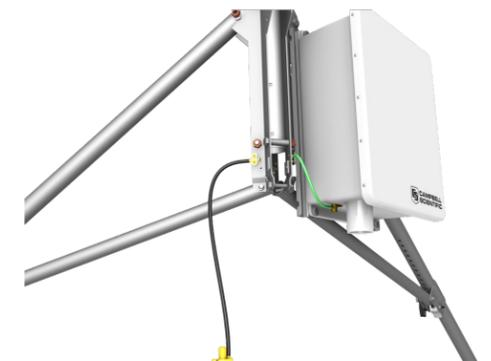
3. Attach the CM20X crossarm to the tripod mast.
