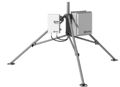
2. Ground the tripod and enclosures.
