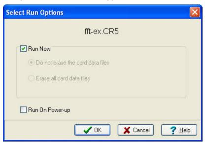
When Run Now is checked, the program is compiled and run in the datalogger. All data tables on the CPU are erased. You have the option of whether or not to erase data files stored on a card.
