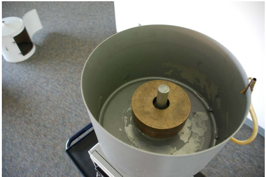
FIGURE 3.4-1. Calibration weights properly placed in the center of the basin.
